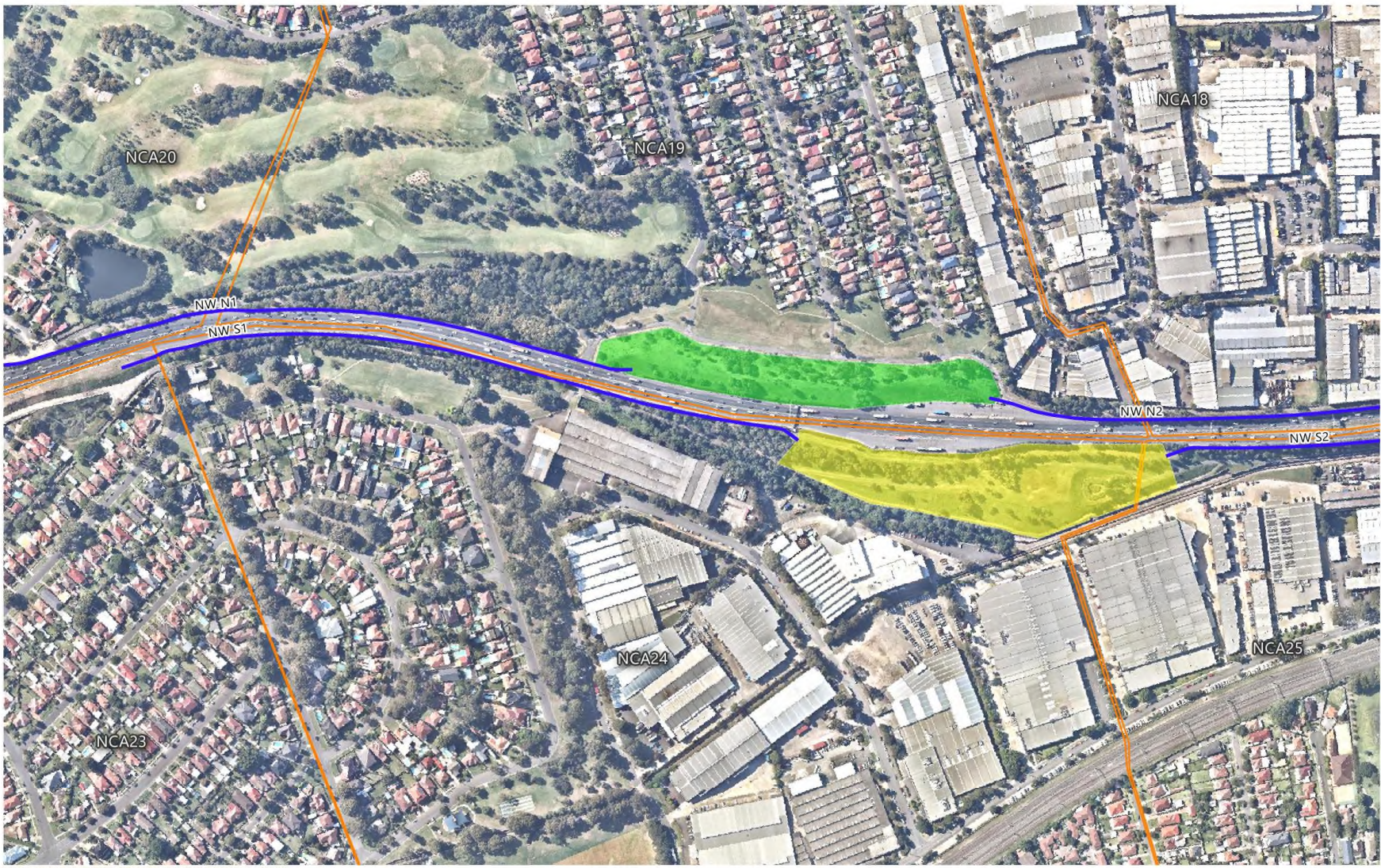
Figure 1 Existing noise walls and mounding
