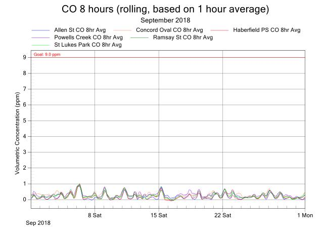
Figure 2: M4 East Project Air Monitoring Stations - CO 8 hours Rolling graph for September 2018
