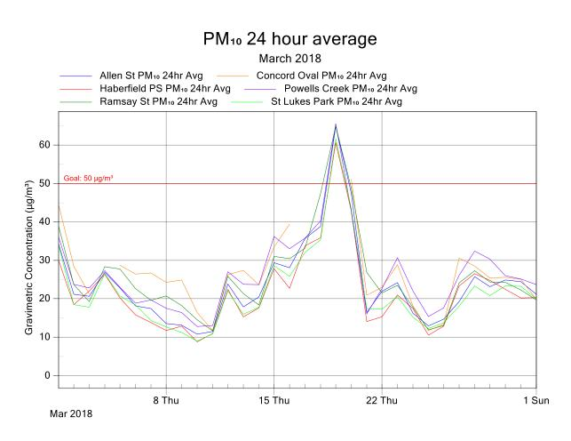
Figure 4: M4 East Project Air Monitoring Stations - PM<sub>10</sub> 24 Hour graph for March 2018
