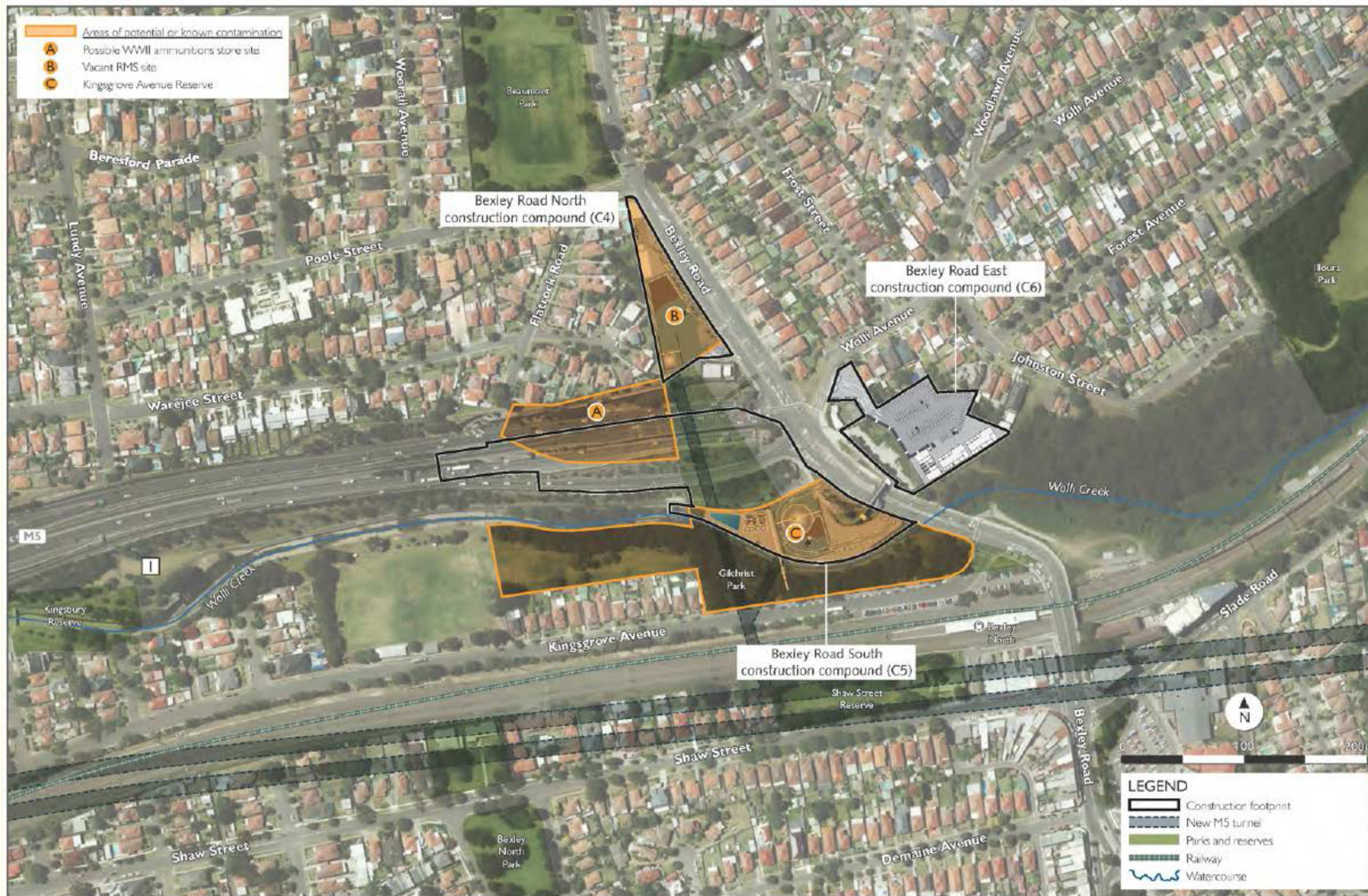
Figure 4b Potential known areas of contamination – Bexley Surface Works
