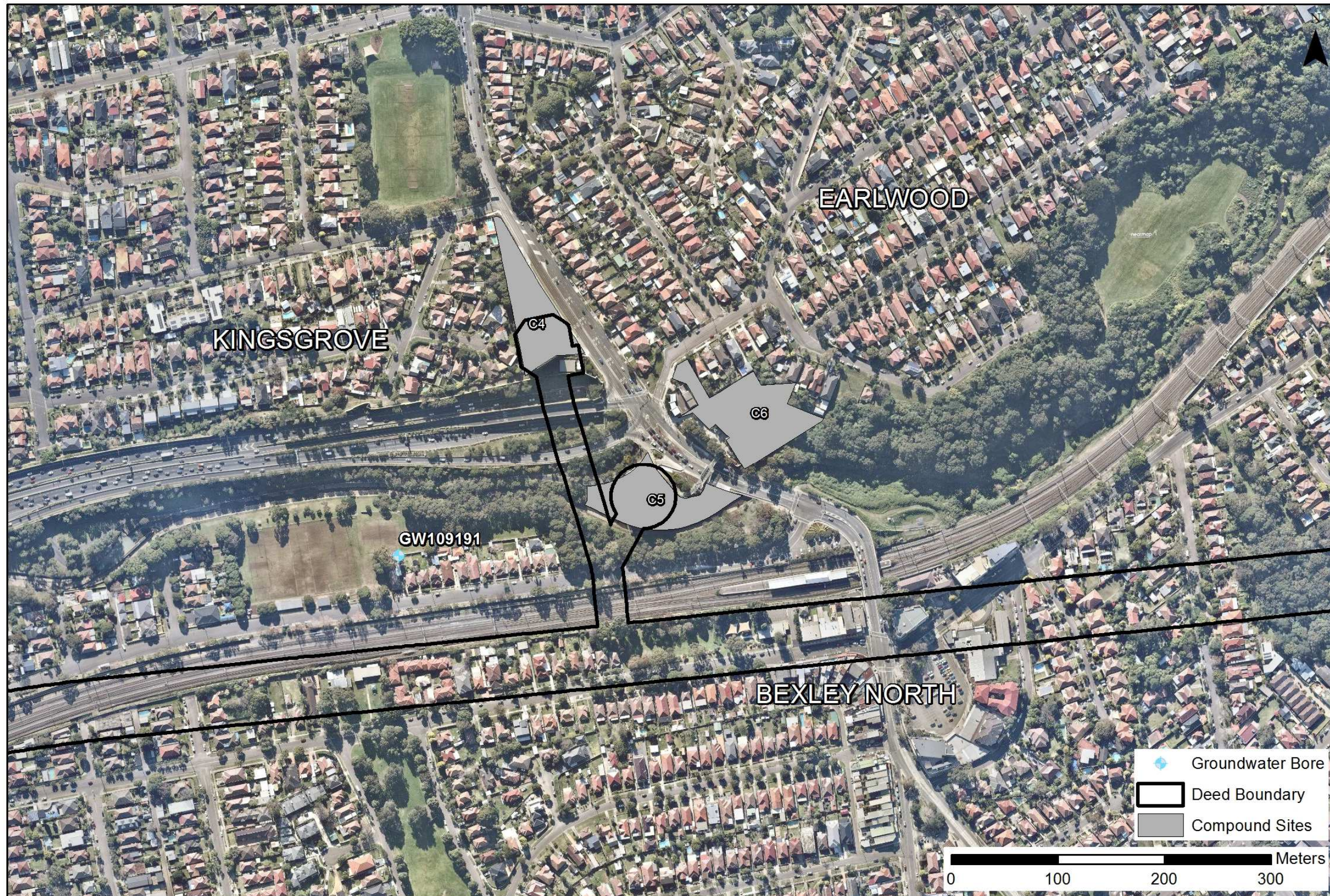
Figure 5c: Location of groundwater bores that may potentially be affected by tunnelling - Bexley Surface Works
