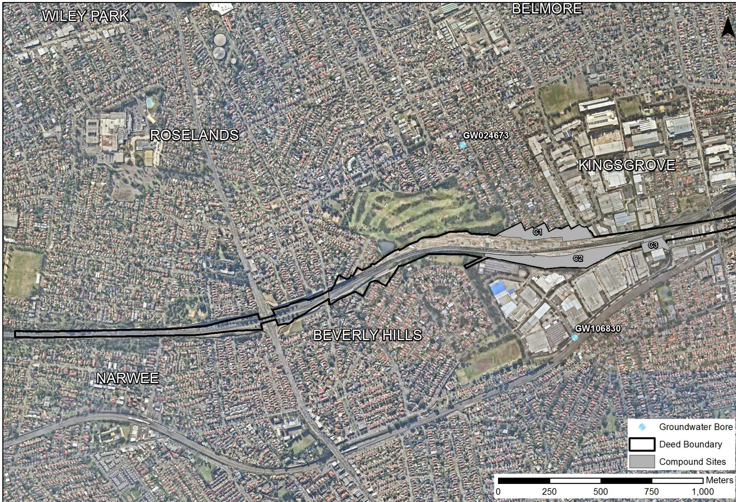
Figure 5d: Location of groundwater bores that may potentially be affected by tunnelling - Western Surface Works
