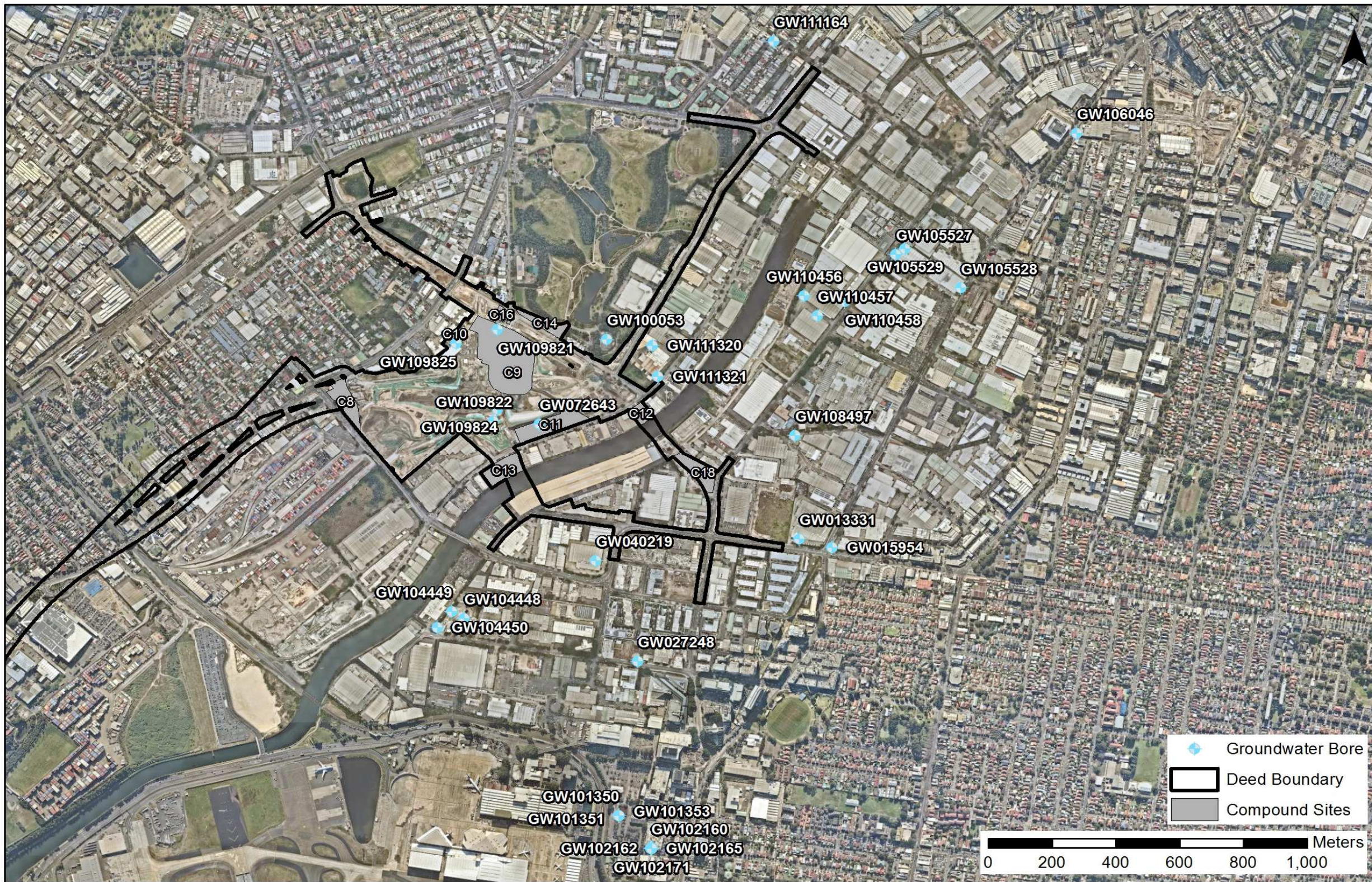
Figure 5a: Location of groundwater bores that may potentially be affected by tunnelling - St Peters Interchange and Local Roads Upgrades
