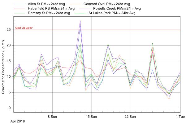
Figure 5: M4 East Project Air Monitoring Stations - PM<sub>2.5</sub> 24 Hour graph April 2018
