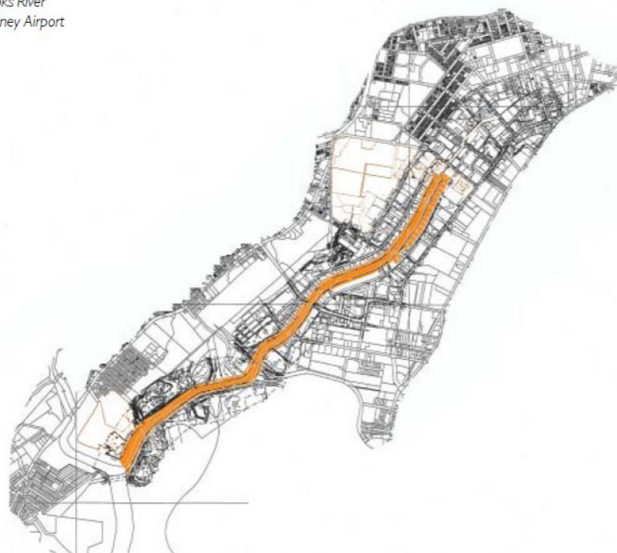
Figure E-31 - The curtilage of Alexandra Canal based on the Conservation Management Plan prepared by the Government Architects Office of NSW, establishes a minimum distance of 3 metres either side of the top of the canal wall. The curtilage is shown as an orange line on the adjacent image.
