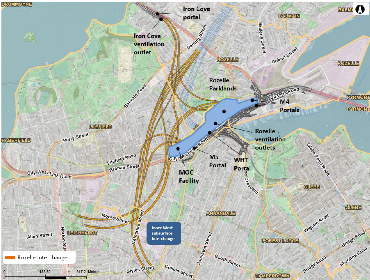
Figure 2-1: Key features of the Asset as upgraded under the approved project
