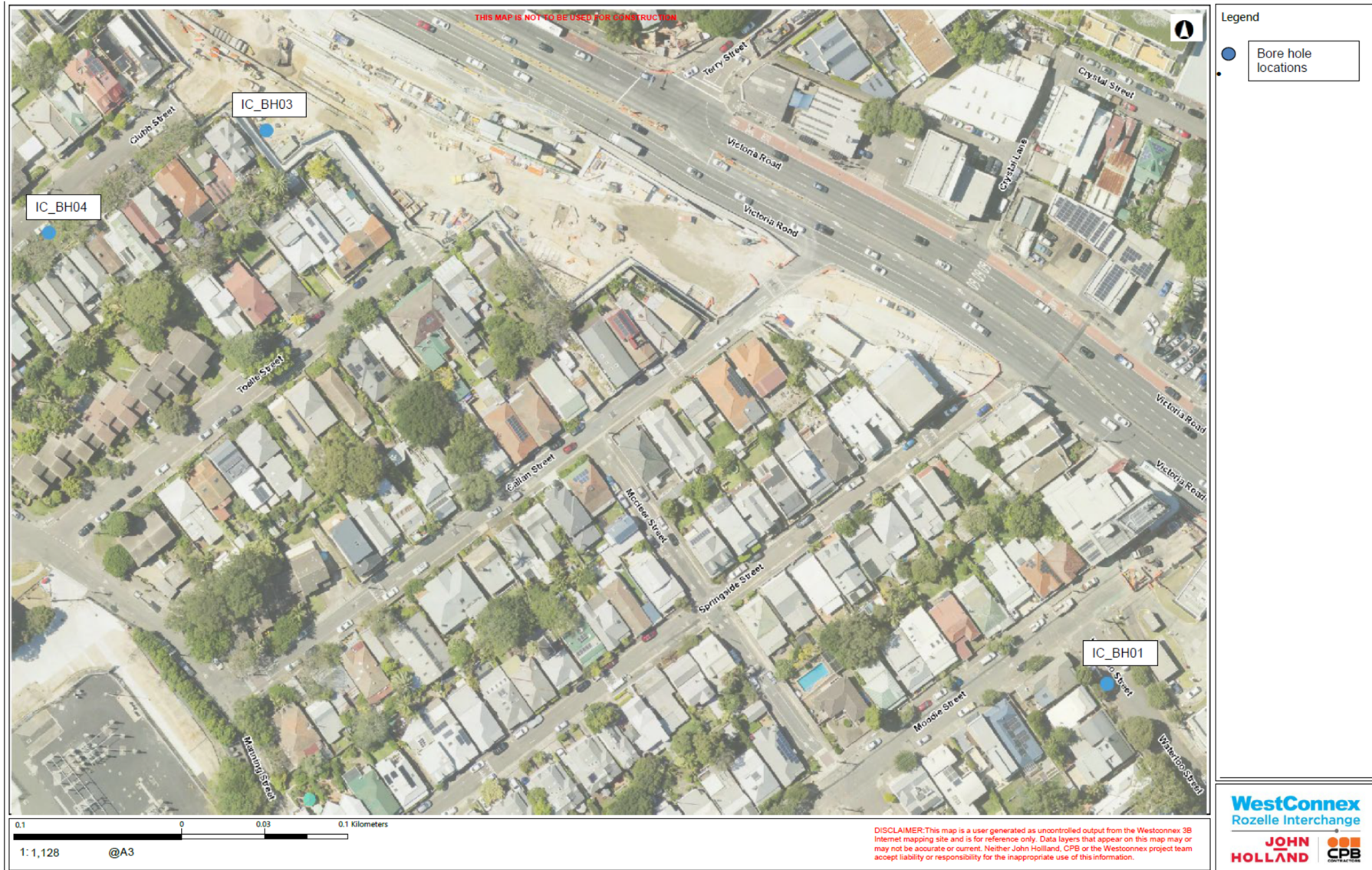
Figure 4 Operational phase groundwater monitoring network – salinity logger locations (Iron Cove)
