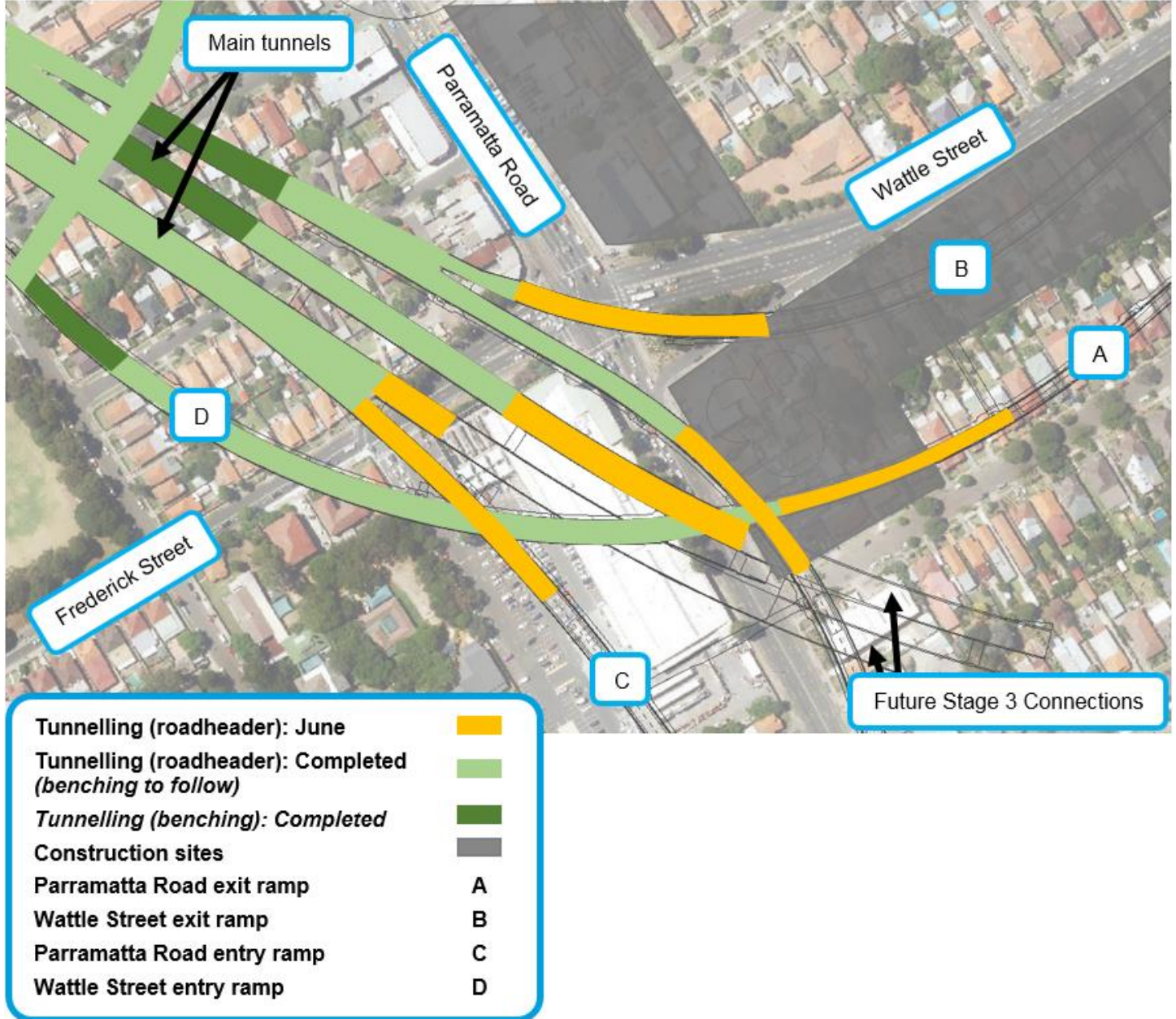
Location of tunnelling activity – Northcote Street construction site.
