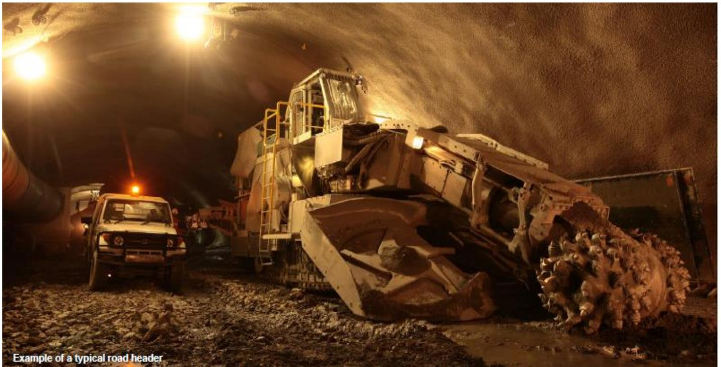
Example of a typical road header
